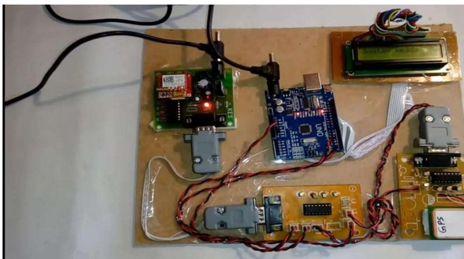
The vehicle tracking system works mainly by receiving messages from a mobile phone. There is a message command by which we can track the vehicle. And this command is to send an SMS; "TRACK VEHICLE" to the registered SIM card number in the GSM modem. This command initiates the GPS modem and receives the latitude and longitude position and this information will then be sent as SMS to the mobile device.
