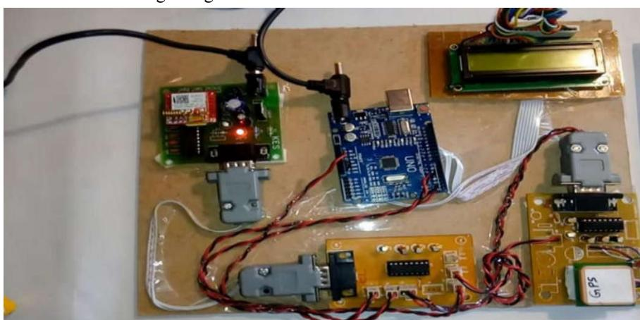
When power supply is given to the device through two 9v adapters to the arduino and GSM, then the system shows ready on the LCD display to track the location.
