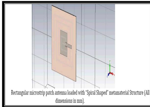
**Figure.2:** metamaterial structure
