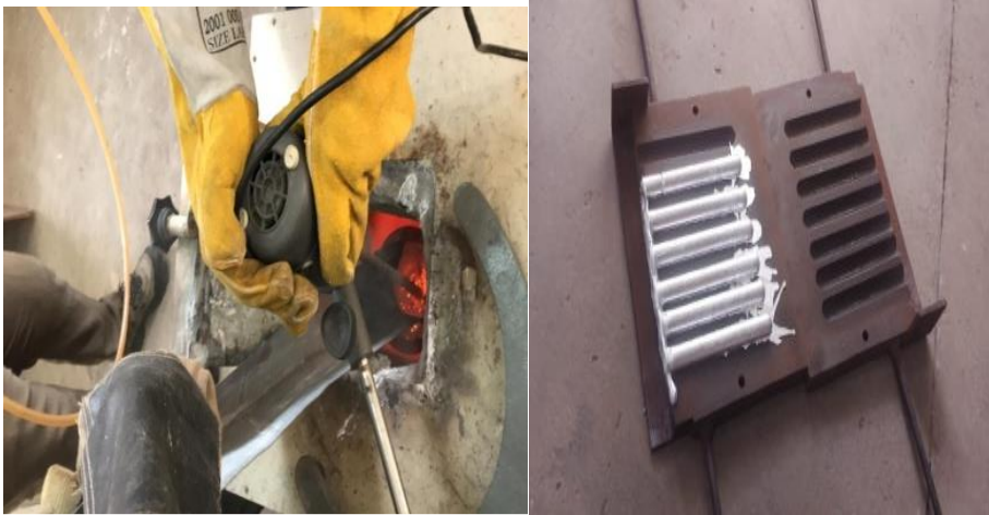
Figure: Stir casting - Cast fingers
