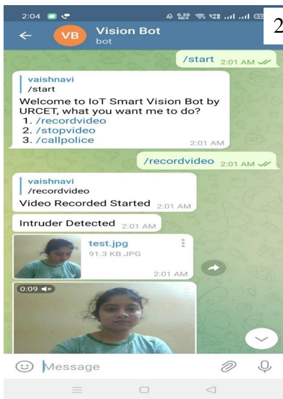
Figure: Intruder detected notification through telegram bot
