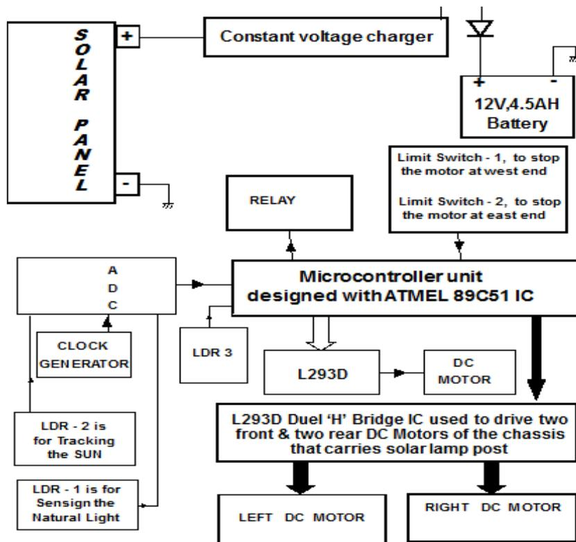
2) In this paper two LDR's are used, the first LDR is used for detecting the intensity of sun light, for energizing the system and the second LDR is used for detecting the position, to drive the panel towards the sun direction.
